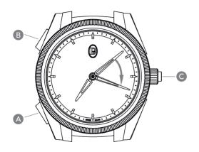
When using the split-minute function, as soon as you press either push-piece A or B, the split-minute hand will detach from the minute hand, and remain fixed. If you make a time setting when the split-minute hand is active, it will remain in its set position, with only the conventional hour and minute hands moving.
